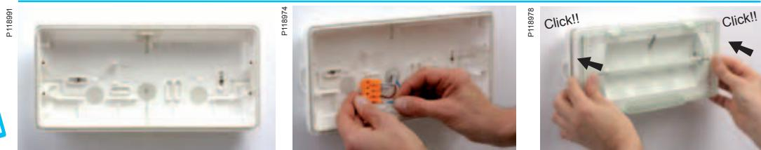
The body can be pre-installed so that the light fitting then just clicks into place. Screwless connector 2 x 2.5 mm<sup>2</sup> per input.
